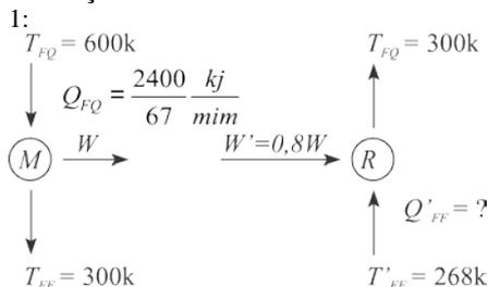
$$\eta_{motor} = 1 - \frac{T_{FF}}{T_{FQ}} = 1 - \frac{300}{600} = \frac{1}{2}$$
