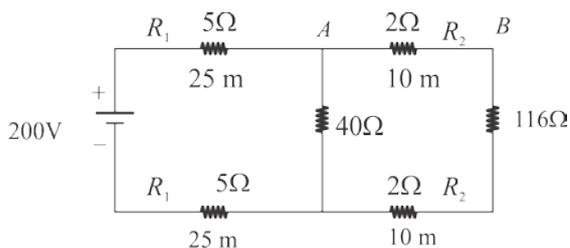
$$R_1 = \frac{\rho \cdot L_1}{A} = \frac{0,4 \cdot 25}{2} = 5\Omega \text{ e } R_2 = \frac{\rho \cdot L_2}{A} = \frac{0,4 \cdot 10}{2} = 2\Omega$$
